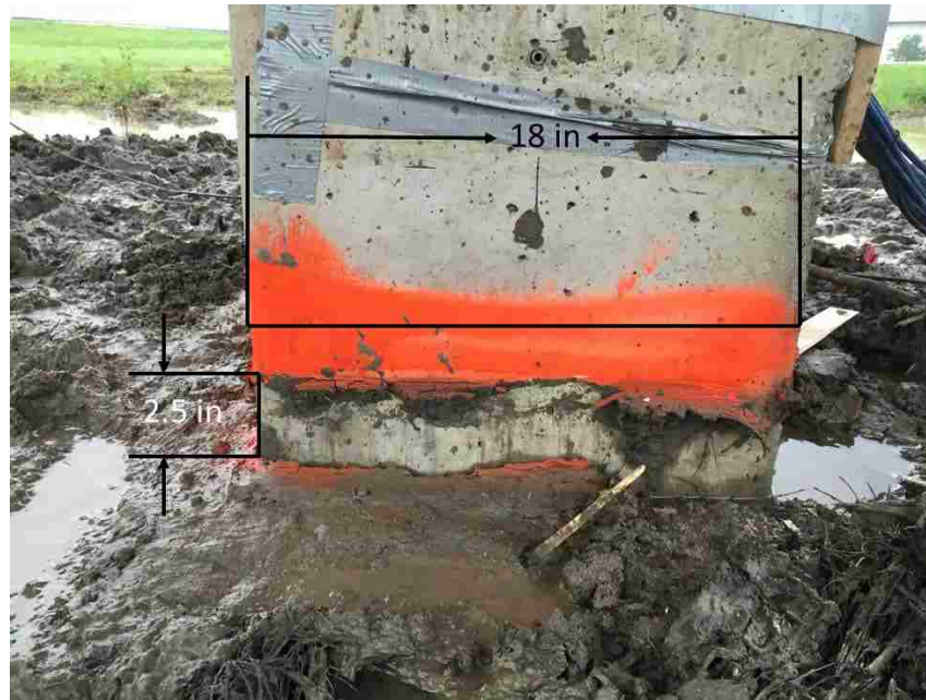
Figure 5.4-5 Photo showing offset between the pre-stressed concrete pile and the surrounding soil after blast test. The painted pile section was initially flush with the ground surface prior to the blast.
