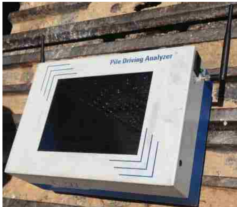
Figure 4.4-2 Pile Driving Analyzer device.
