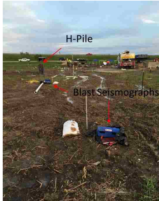
Figure 5.5-3 Photograph of two InstanTel Minimate blast seismographs in place prior to blast liquefaction test around the concrete pile.
